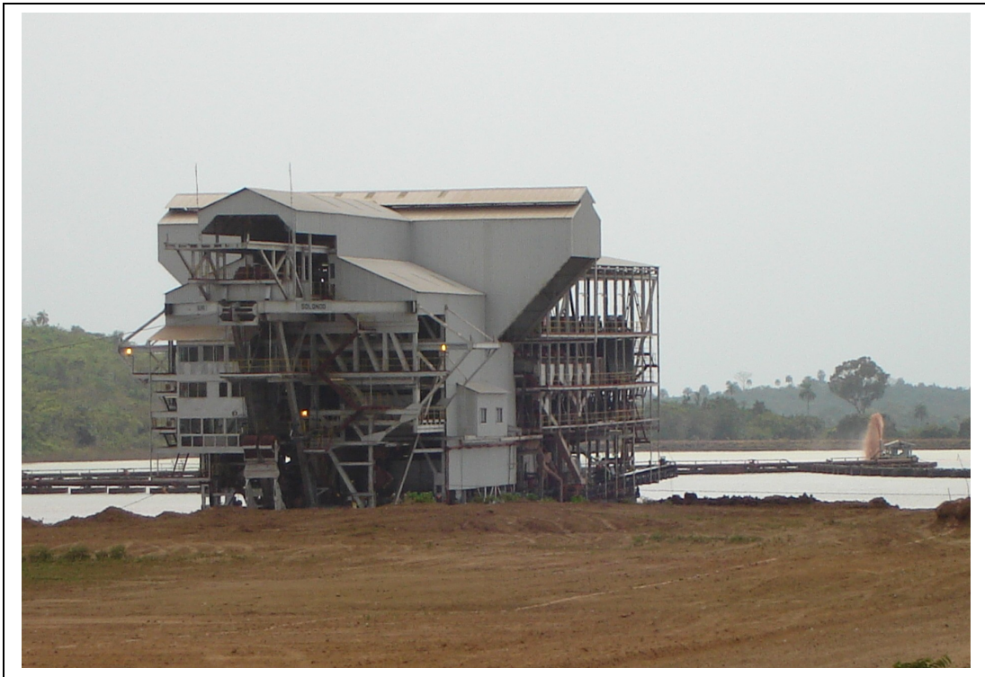
At work Solondo eating the land away and sending sand tailings and slime back into the pond
